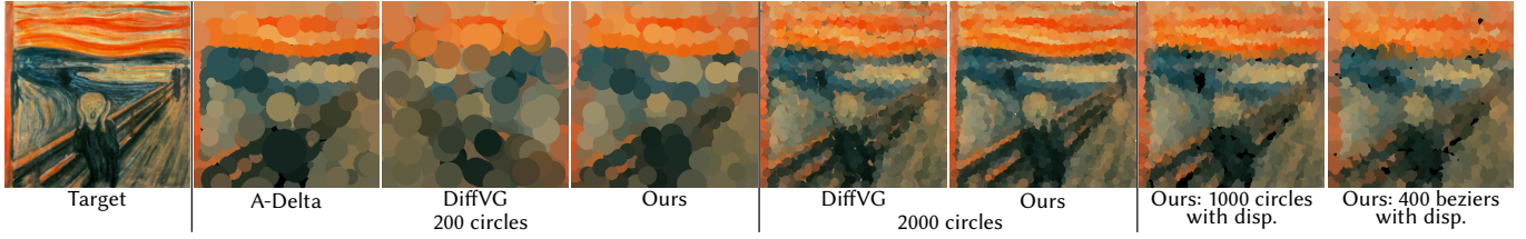
Fig. 12. Painterly rendering . Given a target image (left), we optimize a set of randomly initialized primitives using an L_2 loss to produce a painterly renderings. With 200 circles, all methods capture the rough structure of the target. With 2000 circles, both our method and DiffVG produce painterly renderings with lower reconstruction error, while A- \delta does not scale to the large number of primitives (Fig. 13). Unlike DiffVG, our method does not require specialized boundary sampling routines; it supports non-standard primitives like noise-deformed circles and bezier curves (final two columns).
