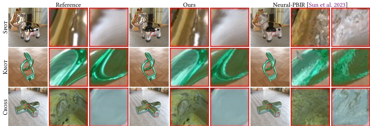
Fig. 10. Comparison against Neural-PBIR [Sun et al. 2023] on glossy object reconstruction. We evaluate the quality of glossy object reconstruction using Neural-PBIR and our method. Due to the fact that Neural-PBIR’s initialization stage often fails for glossy objects, we specifically evaluated the mesh refinement stage. In this experiment, we start with the same initial geometry obtained from a visual hull and compare the physics-based inverse rendering (PBIR) mesh refinement. Our PBIR-NIE demonstrates superior reconstruction quality, effectively capturing detailed highlights from the environment. In contrast, Neural-PBIR struggles to reproduce glossy materials and geometric details.
