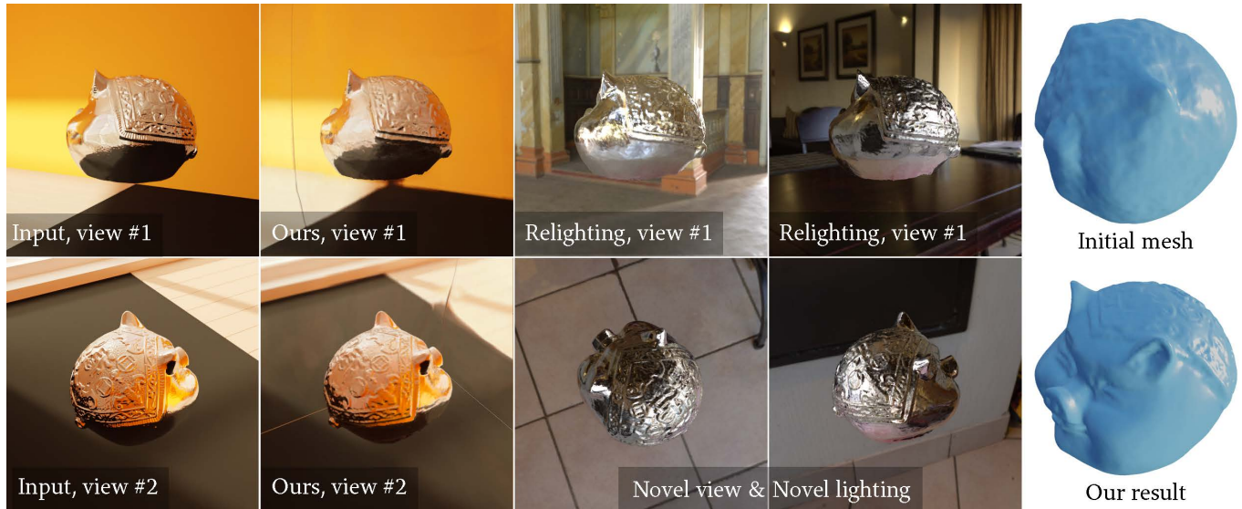
Fig. 1. We propose PBIR-NIE, a physics-based inverse rendering pipeline that optimizes an object’s shape, glossy surface reflectance, and non-distant lighting representation. Our method faithfully recovers the shiny and specular appearance, produces relighting results with high fidelity, and accurately captures geometric details from a rough visual hull initialization.
