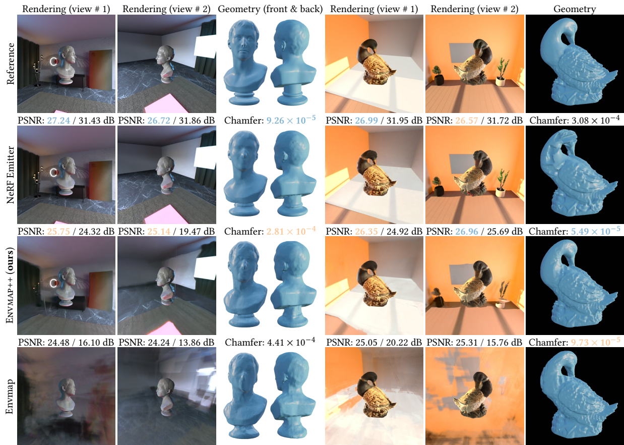
Fig. 11. Comparison of lighting representations: NeRF Emitter [Ling et al. 2024], our ENVMAP++, and standard environment map. In these two scenes, we jointly optimize the object shape, materials, and surrounding lighting with each lighting representation. We report the quantitative results — PSNR for the foreground-only region and the whole image (in the format 'PSNR: (foreground / whole) dB'), as well as Chamfer distance — above the corresponding image, and color-code the best and second best method accordingly. Our pipeline successfully recovers the object's geometry, while the standard environment map fails in these scenes due to the violation of the infinite-distance assumption and background parallax. NeRF Emitter uses a NeRF for background lighting, which is computationally expensive. In contrast, our ENVMAP++ is a lightweight representation, providing more efficient inverse rendering optimization.
