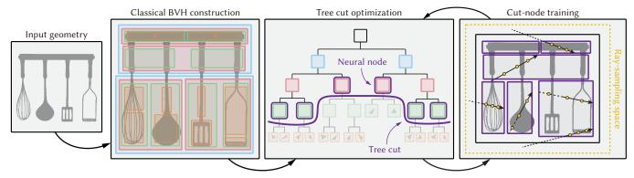
Figure 2: Our lightweight N-BVH is a shallow hierarchy whose leaf nodes simply store bounds within which we search for ray intersections by querying a neural geometry representation. The leaves (in purple outlines) represent a cut in a classical BVH over the input geometry; we optimize the cut by iteratively splitting the leaves with largest inference error. After each splitting step we train our neural model within the cut-node bounds by sampling random rays in the scene.
