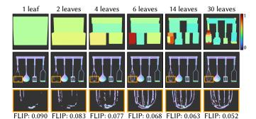
Figure 5: Increasing the number of N-BVH leaf nodes consistently improves the reconstruction quality. It also improves performance on this scene with low depth complexity where at most one neural inference per ray is needed. The top row visualizes the average training loss per node in false color.
