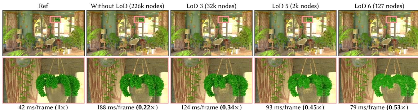
Fig. 5. Primary ray intersection LoD switch. We train our \mathcal{N} -BVH for a total of 7 levels of detail, each corresponding to a different number of nodes in the learned tree cut. We then render using the most detailed LoD for primary rays, an one of the coarser LoD for secondary rays. For finer LoDs the perceived error only slightly decreases while already providing a drastic speed-up. For coarse LoDs, close-up renders reveal missing shadows on high-frequency geometry but still provide a solid approximation in the distance.
